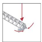
**A1:** The lattice girders are clamped into the fibre concrete spacer (3 pieces per girder)
