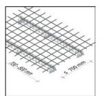
**A3:** Observe maximum installation distance between lattice girders and fibre concrete spacers
