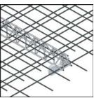
**B3:** Observe maximum laying distance. Put on upper reinforcement.
